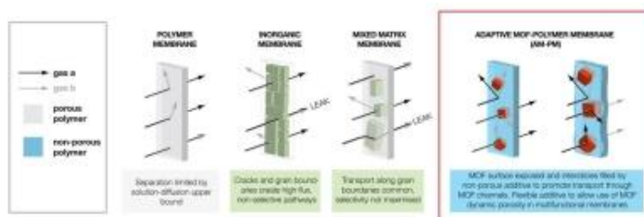
Figure 1 - Comparison of the proposed membrane architecture compared to current organic, inorganic and mixed matrix membranes.
