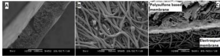
Figure 2. A) Cross section of a membrane with spongy structure; B) Fiber mesh morphology obtained by electrospinning; C) Cross section indicating the tight adhesion between membrane and fiber mesh.
