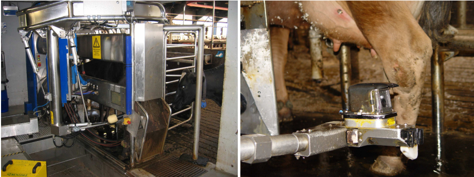
Figure 2.6: An automatic milking system.
