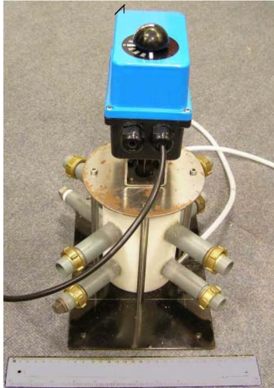
Figure 12: Prototype of 8-way valve operating with a \frac{1}{4} turn fast electrical actuator (1 second)
