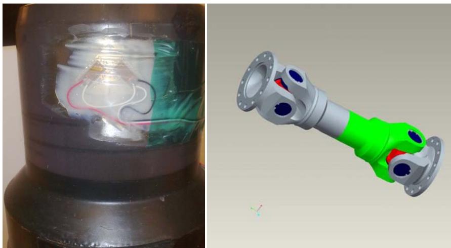
Figure 16: Details of the torque sensor installation (left) on the cardan joint (right)
