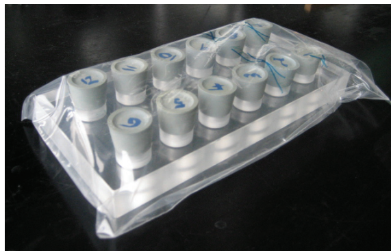
Figure 8.6 Photo of the PMMA block used for assessing the influence of strontium on the BMD results in Sr-rich bones. The DEXA measurements were performed with the rubber stoppers removed.
