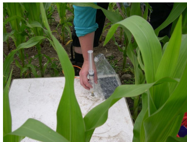
Emission of N 2 O was measured by manual gas sampling in gas-flux chambers
