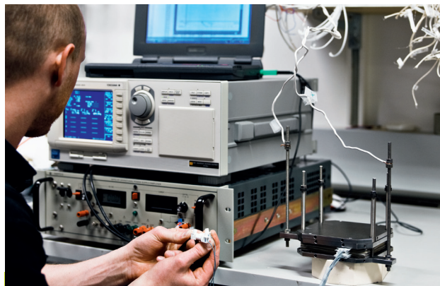
Detailed characterization and testing is essential to develop advanced ceramic components. Unique test facilities ensure that advanced tests can be performed on both individual components, cells and (as shown here) stacks of cells.
