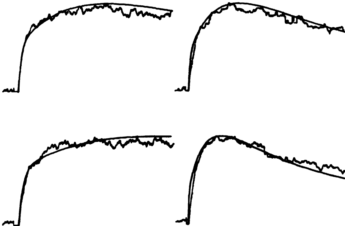
Figure 6.16. Comparison between experimental and computer simulated HS-kinetics in H 2 S/Ar-mixtures. Normalized absorbance vs. time. Lower left: 1 mbar H 2 S, upper left: 2 mbar H 2 S, upper right: 5 mbar H 2 S, lower right: 10 mbar H 2 S. Total pressure = 1 atm.
