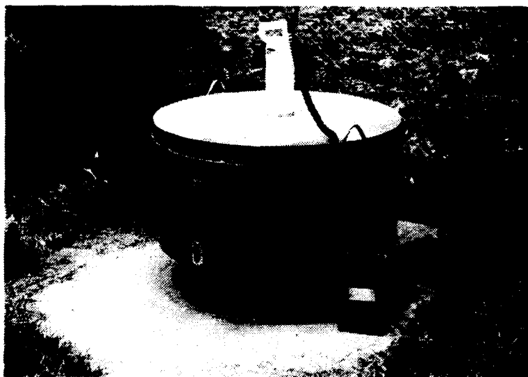
Fig. 25. Portable GR-410 spectrometer set up for monitoring of small calibration pad at Villa 25 de Mayo in the Mendoza province, Argentina.
