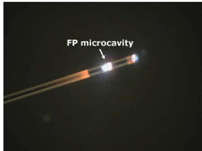
FIG. 2. (Color online) Microscope image of the light guided in a \sim 500 \mu\text{m} long fiber taper with the FP microcavity and the shattered fiber end.
