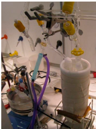
Figure 44. Photograph taken during oxidation of sample formic acid. The U-tube in the foreground is submerged in liquid nitrogen in a dewar to trap carbon dioxide. The reaction flask which is seen in the background with the reflux condenser (blue tubes).
