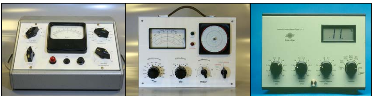
Three different versions of the Comfort meter, developed by Thomas Lund Madsen. The one to the right was in production at Brüel&Kjær.
