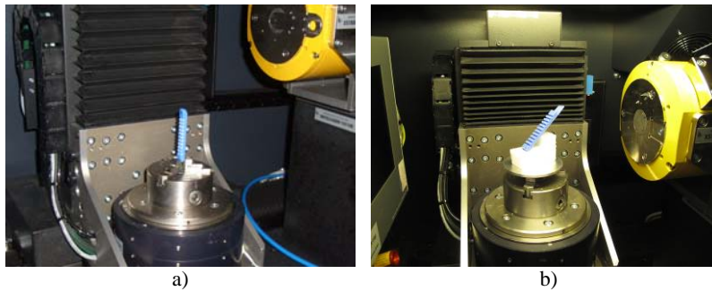
Figure 1: Orientation of the step gauge in the scanner cabinet: a) vertical position; b) inclined 45° with respect to the rotation axis.
