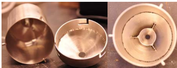
Fig. 6: The platinum crucible main body and lid (left); the inner cone of the gas inlet (right).
