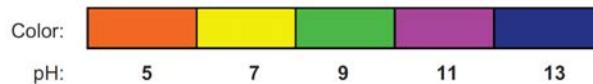
Figure 4.20 Color variations indicated by Rainbow Indicator as a function of pH, from [Instruments].
