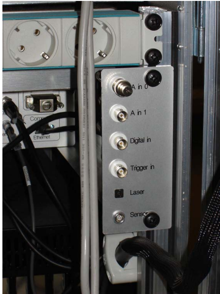
Figure C.14 Channels for input of external signal sources. (Author's photos)
