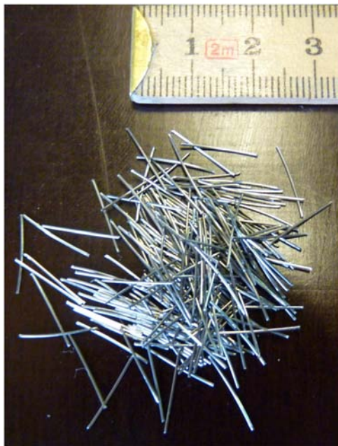
Figure B.4 Steel fiber used for Mixture 2. (Author's photos)
