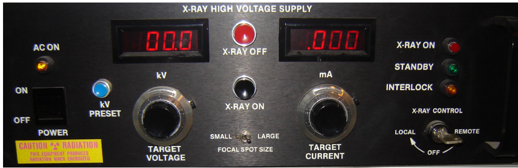
Figure D.11 Control panel for manual operation of the X-ray system. (Author's photos)
