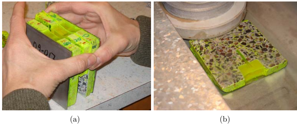
Figure 2.10 (a) WST specimen were sliced in 3 pieces after fluorescent epoxy impregnation. The outer slices were impregnated again from the cut surface to highlight isolated microcracks and (b) were ground to remove excess epoxy. (Author's photos, taken at Pelcon Materials & Testing ApS)
