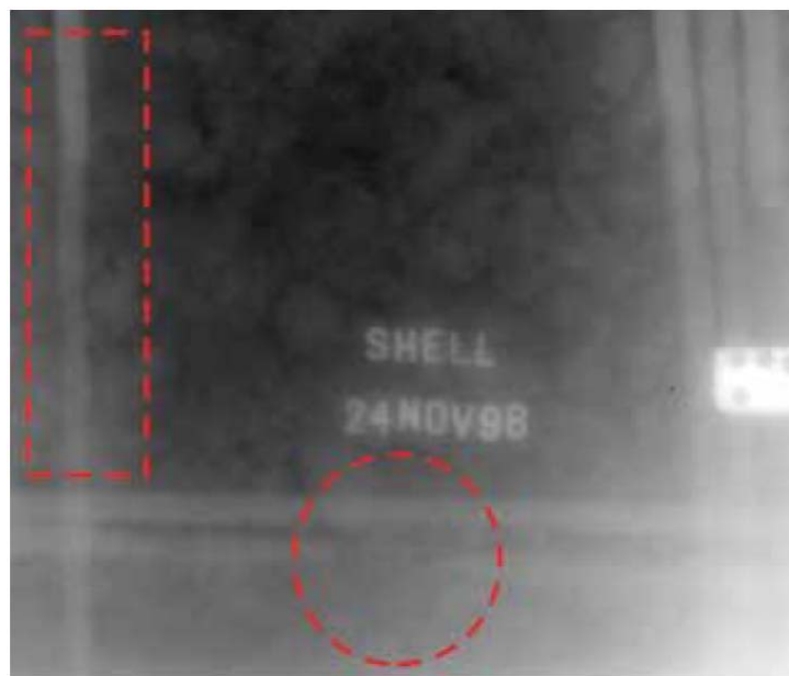
Figure 4.14 \gamma -ray image with areas of severe corrosion indicated in red [Mariscotti et al. , 2009].
