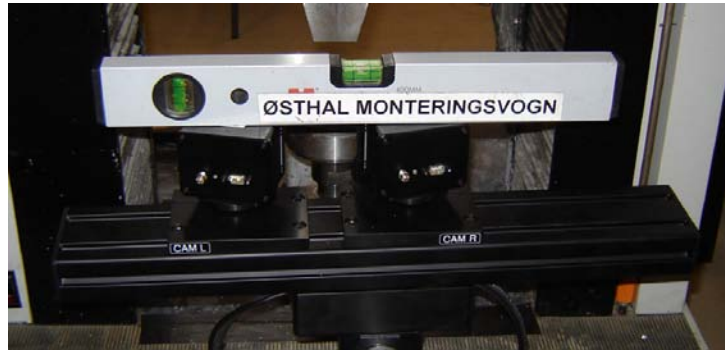
Figure C.4 Insuring cameras are on level plane. (Author's photos)
