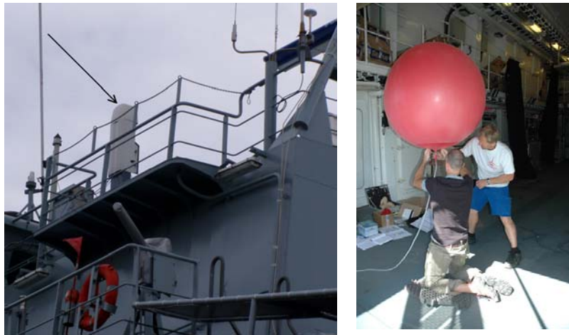
Figure 6.1. Left panel shows the ceilometer (arrow) mounted on the research ship Galathea. Right panel shows the preparation of a radiosounding during the Galathea expedition.
