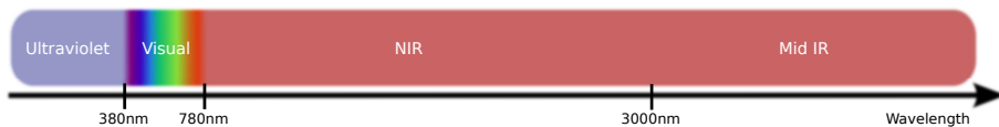
Figure 2.1: The electromagnetic spectrum of the infrared range (IR) above the visual region (cf. ISO20473). Other IR range divisions exist, eg. CIE and DIN.
