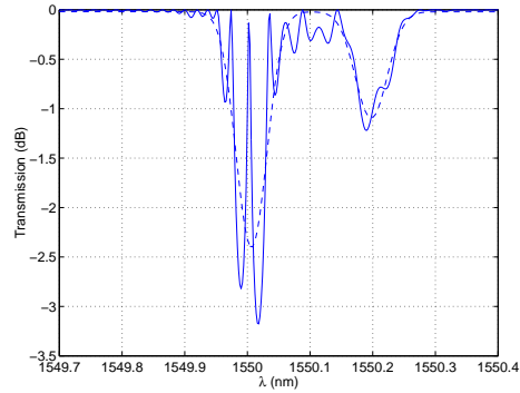
Figure 5.29: The simulated transmission spectrum for a sample with a n_{avg} as illustrated in Figure 5.28. The dashed curve represents the fitted function.
