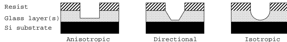
Figure 3.6: A schematic illustration of the different etching profiles possible using a RIE.
