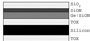
Figure 3.11: A schematic illustration of a UV written sample with a trapping layer made from SiON.
