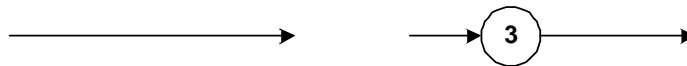
Figure 2.2: Two different representations of a connection, to the right the state associated to the stream is indicated by the number '3', which can then be used for reference for example in a table.
