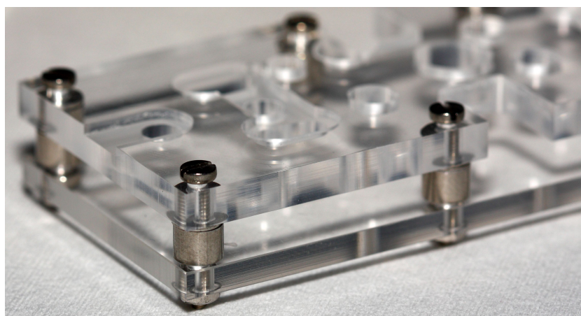
Figure 5.8: The micromilled case is here shown without the chip inside. The metallic cylinders seen around each screw are the spacers. These spacers ensure that the PDMS is compressed in a very reproducible manner
