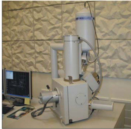
Figure 5.1. The Inspect 'S' Scanning Electron Microscope (SEM), from FEI Company, with a tungsten filament electron source.
