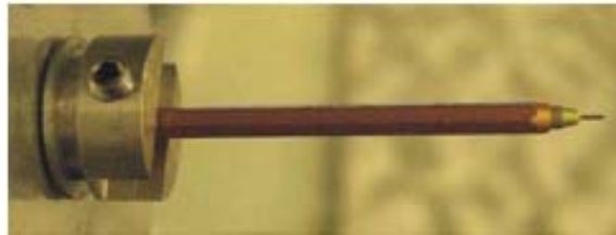
Figure 3.12. Image of a TESA wire gauge, with an external calibrated diameter of 250 \pm 0,15 \mu\text{m} , clamped and fixed on the SEM stage.
