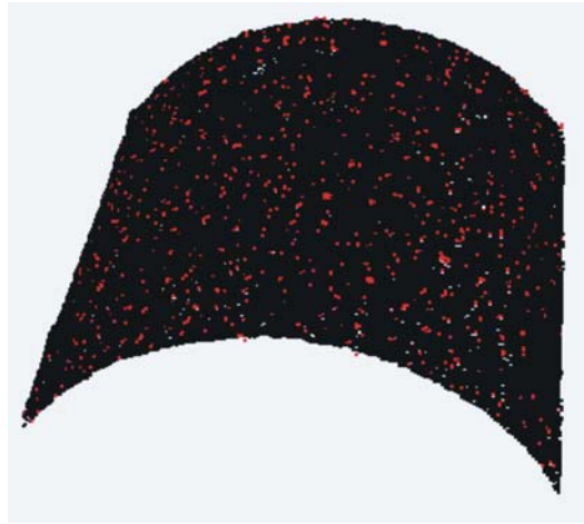
Figure 4.6. Example of a trimmed point cloud showing in red the points suggested being outliers from the Geomagic routine Select Outliers.
