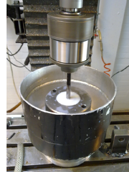
Fig. 2: Clamping of the workpiece and application of lubrication.
