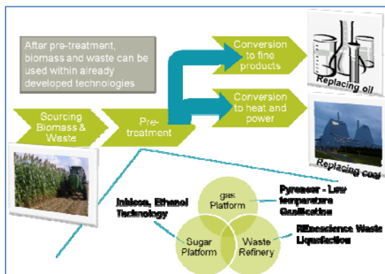
Figur 2 Pre-treatment is a key technology for the utilisation of local biomass and waste
