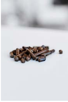
Figure 4: Lignin pellets produced on the INBICON 2G bioethanol plant in Kalundborg.
