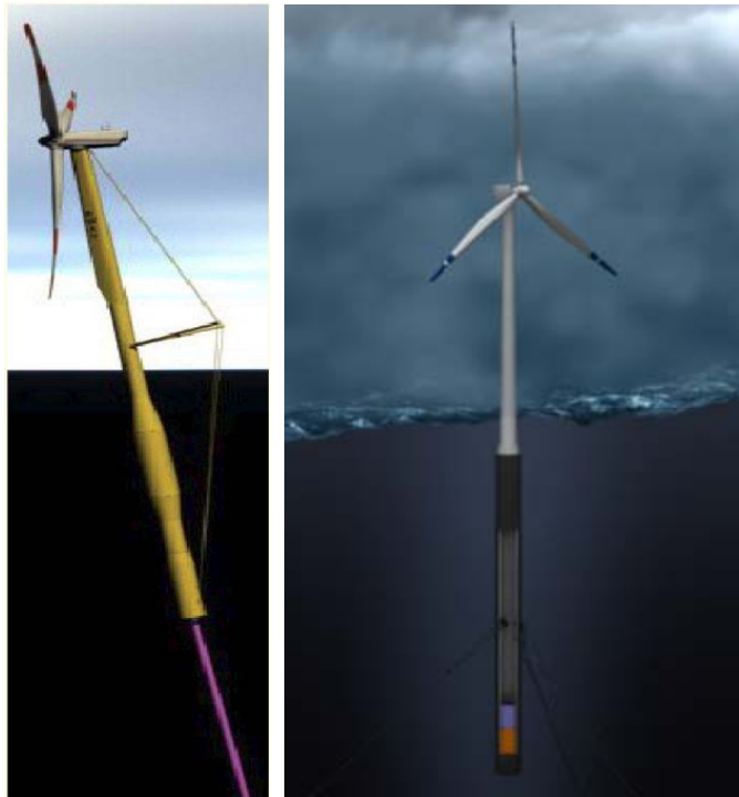
Figure 5: Ideas for floating wind turbines: SWAY (l) and Hywind (r)
