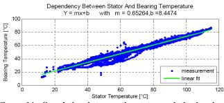
Figure 14: Correlation between the stator and the bearing temperature [6]
