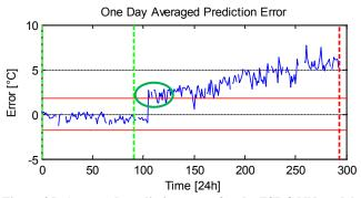
Figure 35: Averaged prediction error for the FSRC NN model
