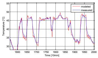
Figure 16: Estimated and measured bearing temperature [6]
