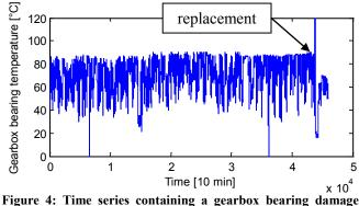
Figure 4: Time series containing a gearbox bearing damage measured on WTG B
