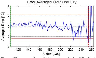
Figure 25: Averaged prediction error of the full signal reconstruction neural network model
