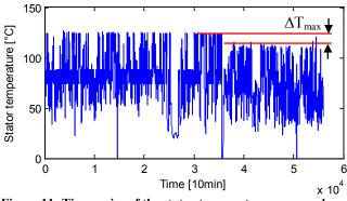
Figure 11: Time series of the stator temperature measured on WTG E
