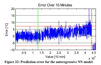
The alarm limit is  $\pm 7.1$  °C. An ALV is first visible 12000 values after the training process has been completed, i.e. 83 days prior to the damage. By this
