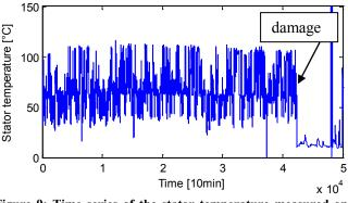
Figure 9: Time series of the stator temperature measured on WTG D
