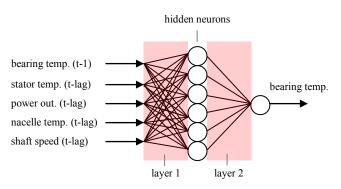
Figure 18: Network architecture - feed forward network [6]
