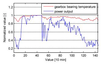
Figure 5: Exemplary power and gearbox bearing temperature fluctuations over time
