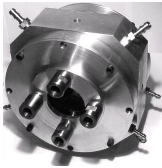
Figure 2.2.1: (a) Scheme of a tilting-pad journal bearing controlled connected to servo valves by means of pipelines; (b) picture of the open bearing with 4 pads and 15 orifices machined on the pad surface; (c) picture of the injectors connected laterally to the pads and bearing housing.
