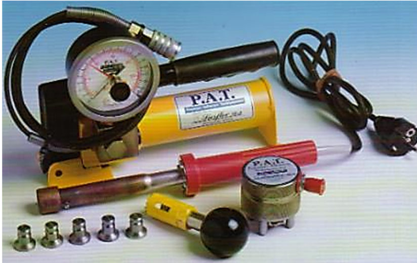
Figure 6.9 The adhesion tester: DFD® PAT model GM01-6.3kN manual hydraulic tensile adhesion tester [16]
