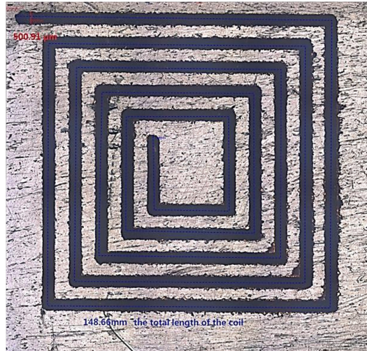
Figure 6.4 One coil sample. The coil was made on polycarbonate (with 10% glass fibre) and plated by copper. The total length is approximately 148mm, and the width of the track is 500 \mu m.
