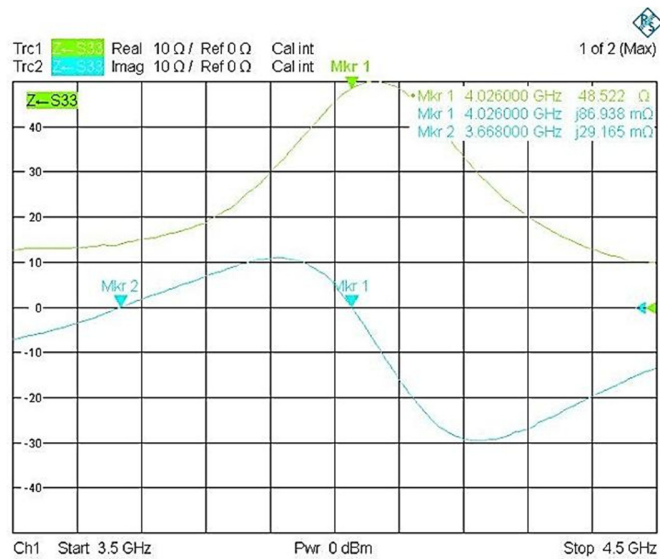
Figure 7.10 Measured input impedance (real and Imaginary) of LISA dipole antenna (3.5GHz-4.5GHz).
