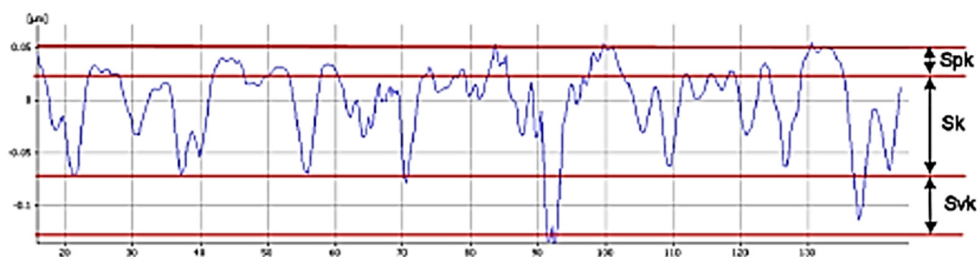
Figure 5.30 Example of the bearing parameters shown by a profile [10][11]
