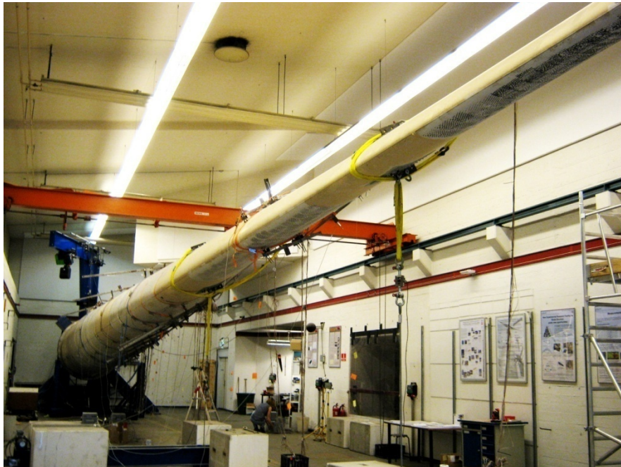
Figure 3.1. Photo of the blade bolted to the test rig. The tip has been cut off, so only 25m is tested. The blade is loaded at an angle of 30° to the flapwise direction, simulating a combined flap- and edgewise loads.
