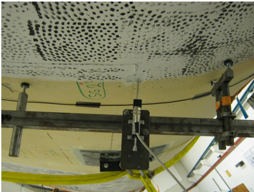
Figure 4.2. Photo presenting the method for placing the LT-NT frames
