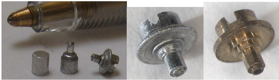
Figure 2.2: Medium complex geometry forged micro part (left and middle) and the machined component (right)
