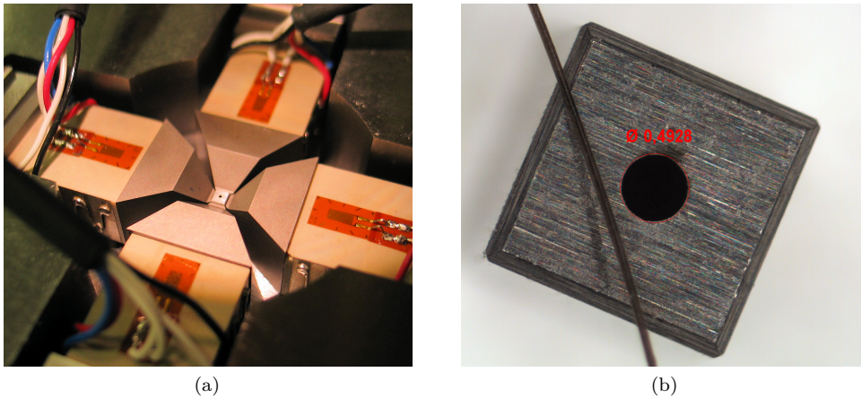
Figure 7.22: Photograph of the dynamic piezo pre-stressing system (a) and a closeup of the small forming die with a overlaid human hair (b)
