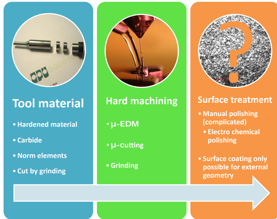
Figure 6.4: Typical processing sequence for a macro scale bulk forming tool
