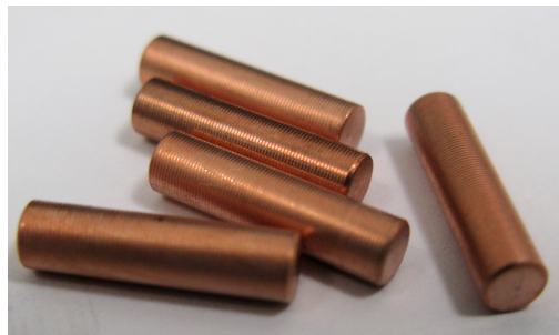
Figure 8.36: Copper coated titanium billets. The copper coating have been applied through electro plating as earlier described. The estimated layer thickness is around 10 μm.
