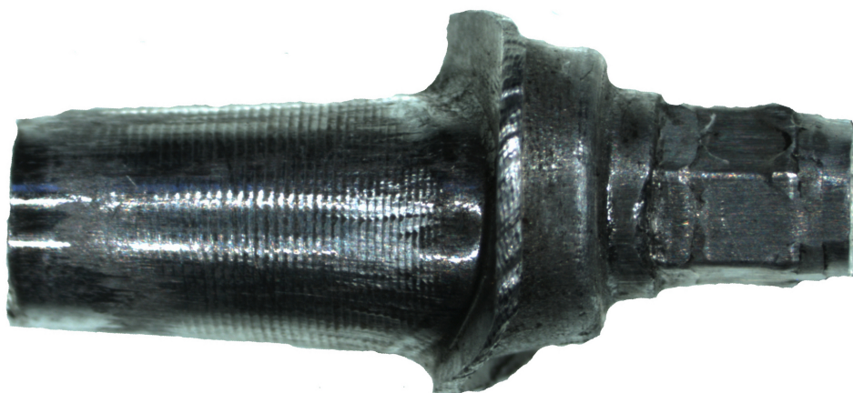
Figure 8.38: First specimen to leave the second forming step. A clear misalignment between the upper and lower forming die is noticeable.
