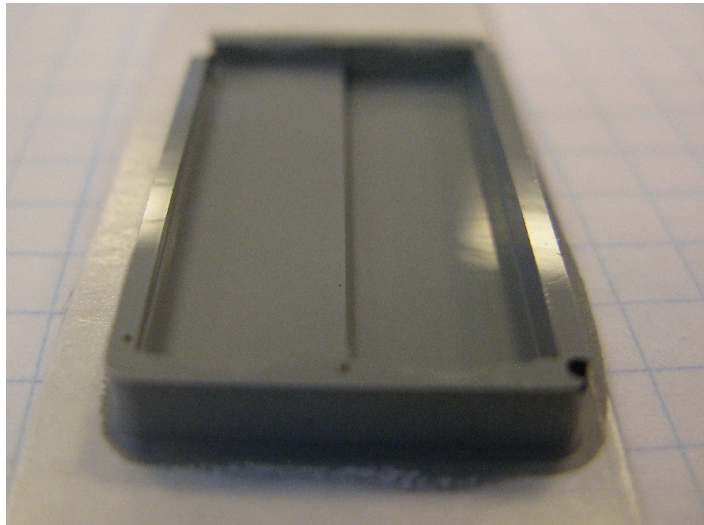
Figure 4.8: Photo of the silicone replica of the step gauge. The Repliset compound GF1 from Struers was utilized.
