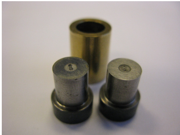
Figure 6.14: Photograph of the manufactured forging dies for micro bulk forming of the cardan axle component. The brass bushing in the background is used for alignment of the two dies during forming.
