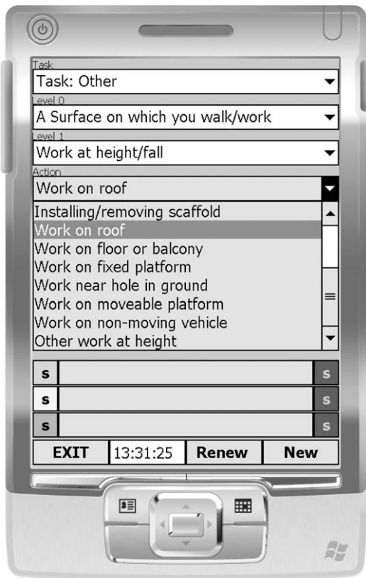
Fig. 3. Example of the PDA interface when selecting an activity to be recorded. The selected activity “working on roof” belongs to group A (surface on which you walk/work), subgroup 1 (working at height/fall). Within this subgroup there are eight possible actions, cf. Table 3.
