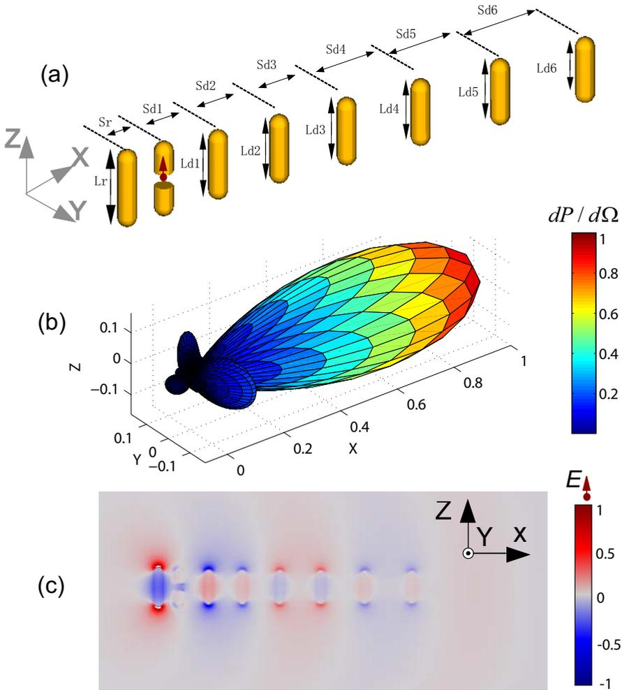
Figure 5.7: (a) Sketch of the nano-optical Yagi-Uda antenna with 8 elements coupled to a quantum emitter. (b) Emission pattern for the emission at  $\lambda=1 \mu\text{m}$ . The emission represents the radiation intensity defined as the power emitted per steradian ( $dP/d\Omega$ ) normalized to its maximum in the forward direction. (c) Snapshot in the  $X-Z$  plane of the  $Z$ -component of the electric field generated by the radiating dipole.
