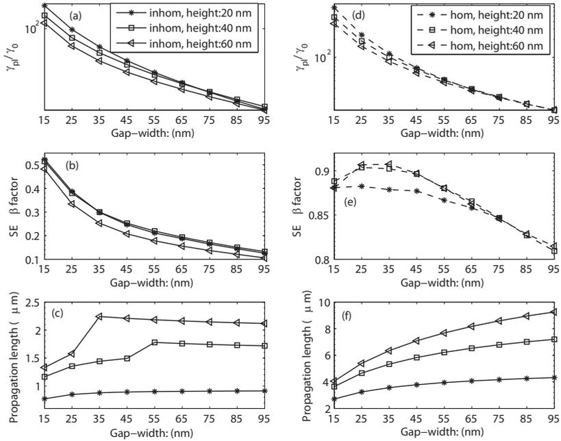
Figure 4.7: Gap-width dependence of the plasmonic decay rates, SE  $\beta$ -factors, and the propagation length of the gap mode for an inhomogeneous dielectric environment (a, b, c) and for a homogenous dielectric environment (d, e, f). In the subplot (a, b, c),  $n_c = 1.5$ ,  $W = 100$  nm and  $n_s = 3.5$ , while for homogenous case in the subplot (d, e, f), the surrounding material is air ( $n_{air} = 1.0$ ), and  $W = 100$  nm.
