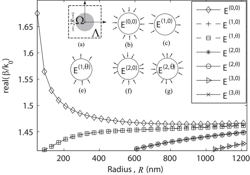
Figure 2.5: Dispersion relation versus radius for the cylindrical gold nanowire with the background medium of PMMA ( $n=1.414$ ) at the wavelength of  $1 \mu\text{m}$ . Inset (a) shows the waveguide structure. Inset (b-g) show electric field orientation of the possible eigenmodes supported by the waveguide.
