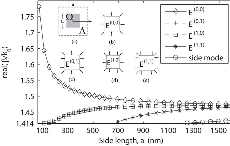
Figure 2.7: Dispersion relation versus side length of square plasmonic waveguides with background medium of PMMA ( $n=1.414$ ) at a wavelength of  $1 \mu\text{m}$ . The metal core is gold. Inset (a) shows the waveguide structure. Inset (b-e) show electric field orientation of the possible eigenmodes supported by square plasmonic waveguides.
