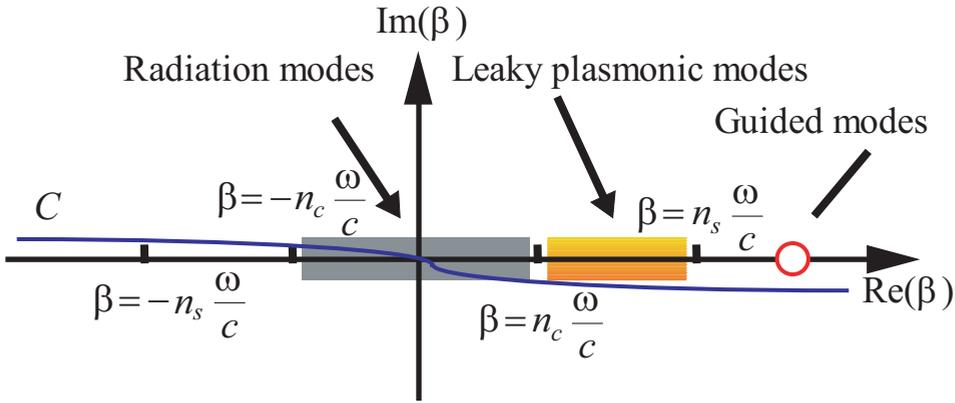
Figure 4.6: Illustration of evaluating the integral representation of the dyadic Green's function. The discrete poles yield the contribution to the decay rates into the guided modes, while the gray and the yellow regions represent the continuum contributions to the radiation modes and the leaky plasmonic modes, respectively. The blue line  $C$  denotes the full integration path.
