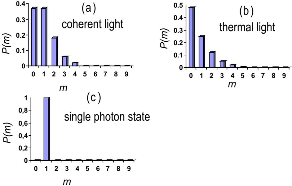
Figure 4.2: Comparison of probability distribution of the number of photons with a mean photon number  $\langle n \rangle = 1$  for (a) coherent light sources, (b) chaotic light sources and (c) the single photon light sources.
