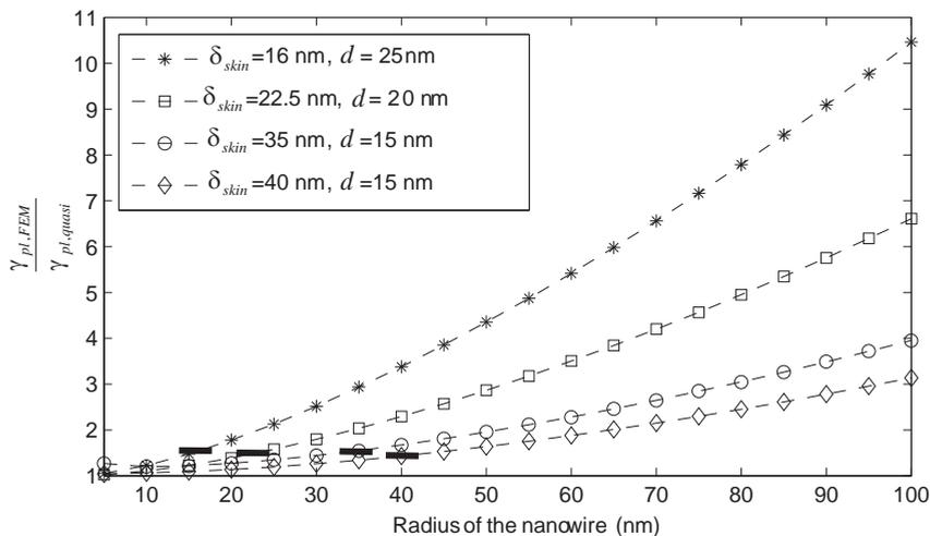
Figure 3.7: The radius dependence of  $\frac{\gamma_{pl,FEM}}{\gamma_{pl,quasi}}$  for four different metals. The skin depths of the four different metals are 16 nm, 22.5 nm, 35 nm, 40 nm, the corresponding relative optical permittivities are  $-100 + 3.85i$ ,  $-50 + 3.85i$ ,  $-20 + 3.85i$ ,  $-15 + 3.85i$ . The vacuum wavelength is  $1\ \mu\text{m}$ .
