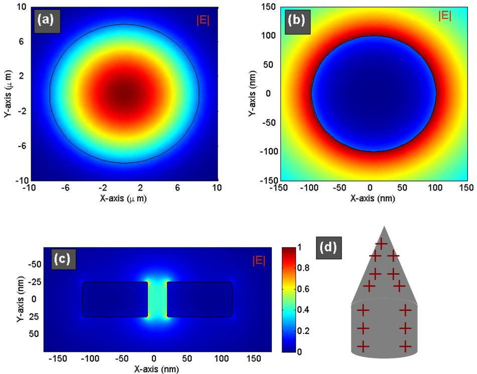
Figure 2.4: Magnitude of electric field  $|E| = \sqrt{E_x^2 + E_y^2 + E_z^2}$  in the transverse plane of (a) the standard single mode optical fiber, (b) 100 nm radius metallic nanowire and (c) the metallic slot waveguide. (d) Sketch of tapered metallic nanowire.
