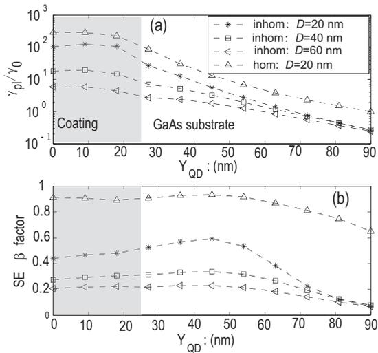
Figure 4.8: Position dependence of the plasmonic decay rates and SE  $\beta$ -factors for the metallic slot waveguide with inhomogenous environment ( $n_c = 1.5$ ,  $n_s = 3.5$ ) and the homogenous case ( $n_c = n_s = 1.0$ ) with  $X_{QDs} = 0$ ,  $H = 40$  nm,  $W = 100$  nm.
