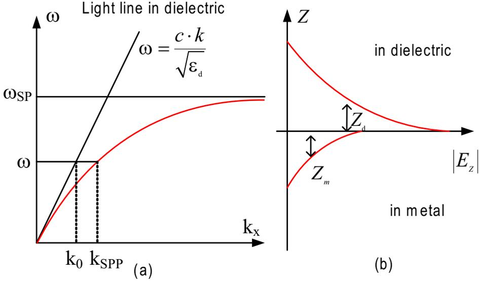
Figure 2.3: (a) The dispersion relation of SPPs at a metallic-dielectric interface. (b) The field profiles of the  $E_z$  component of the SPP in the metals and dielectric.  $Z_m$  ( $Z_d$ ) is the penetration length (field amplitude  $1/e$  length) in the metals (dielectrics).
