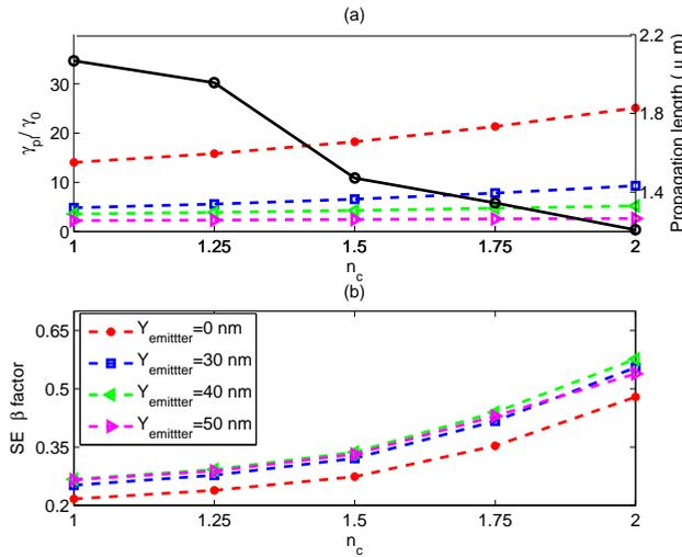
Figure 4.9: Role of inhomogeneous environment, quantified by variation of plasmonic decay rate and SE  $\beta$ -factor with  $n_c$  for fixed  $n_s = 3.5$ ,  $X_{\text{QDs}} = 0$ ,  $H = 40$  nm,  $W = 100$  nm,  $D = 40$  nm. The black line shows the propagation length of the gap mode.
