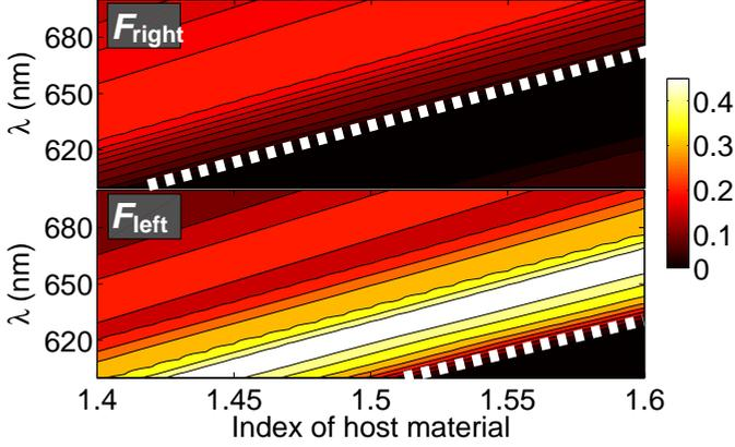
Figure 5.11: Contour plot of beaming fraction  $F$  versus host index and wavelength. The dashed white lines denote the cut-off wavelengths for the directional emissions. In a 30 nm band to the red of the cutoff of the right arms, both beams have comparable power. In between the cutoffs, the right beam becomes extinct, while the left beam becomes brighter.
