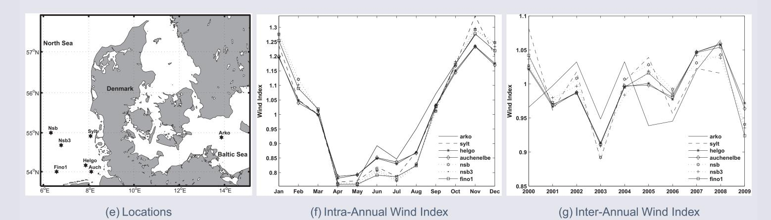
Locations of experimental sites, with platforms and buoys, (left) where Wind Indexes are estimated Intra-annually (middle) and Inter-annually (right) using QuikSCAT data. Wind indexes from in situ measurements will be compared with the QuikSCAT derived ones.
