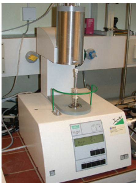
Figure 2.3: The Netzsch STA 449C Jupiter thermobalance.
