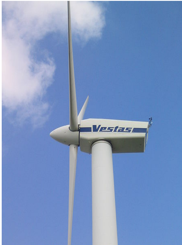
Figure 1.1: Danish-type upwind horizontal axis rotor wind turbine. The three blades are known as the rotor, which is connected to the generator through a drive-shaft, all housed in the nacelle. The nacelle is mounted on top of the tower with a yaw drive enabling the wind turbine to turn towards the wind when the wind changes direction. (Photo by Dirk Ingo Franke and reprint permitted under the CC-BY-SA license.)
