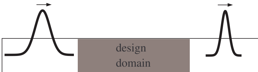
Figure 3: Design problem. A single gaussian pulse is to be compressed when propagating through the design domain by a suitable stiffness and mass density distribution in space and time.
