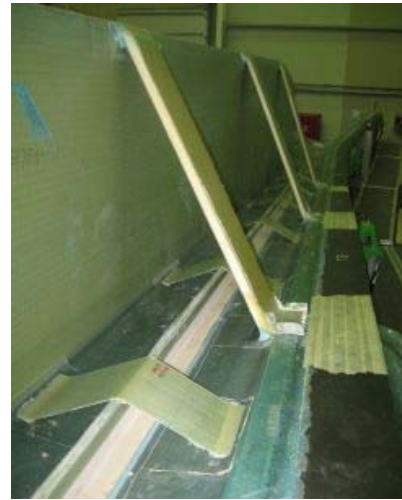
Figure 12. The assembled box girder with cap reinforcement in both upper and lower part and cross reinforcement between the corners.
