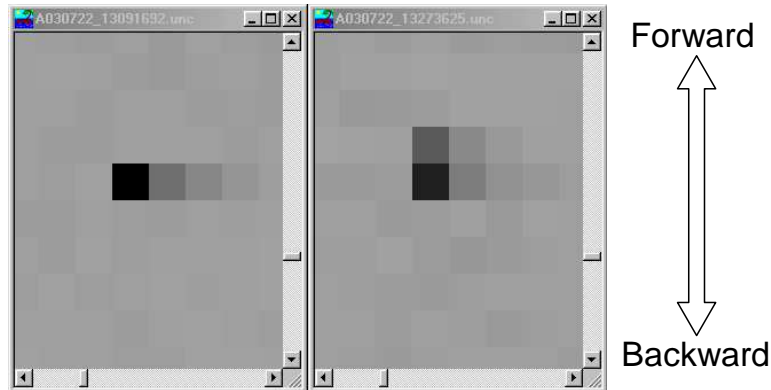
Figure 3.8: Result of backward charge transfer. The left zoomed image part shows an area with integrated charges. In the right zoomed image part a backward motion was exercised leading to a forward smearing.
