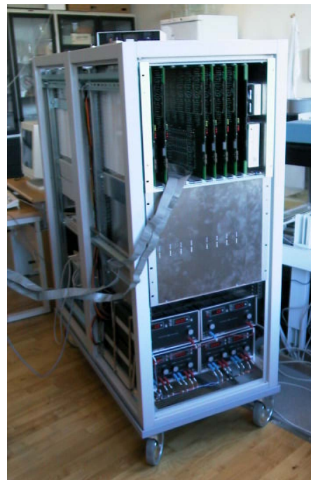
Figure 4: The RASMUS scanner seen from the front with the receivers on the top, transmitters in the middle and the power supplies in the bottom.
