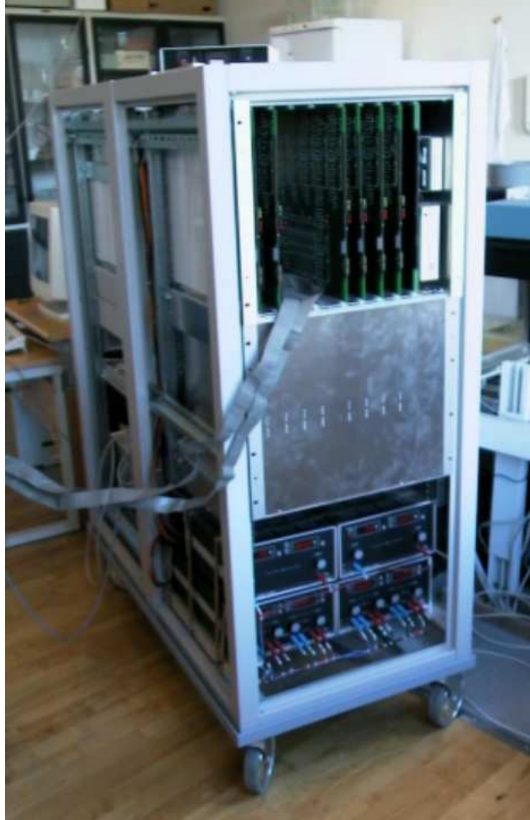
Figure 6: The RASMUS scanner seen from the front with the receivers on the top, transmitters in the middle and the power supplies in the bottom. The analog front-end and transducer connection along with a control PC is placed in the other rack cabinet.
