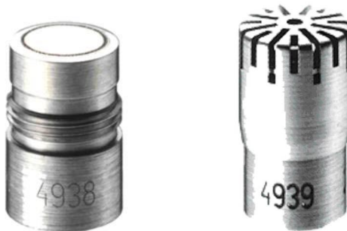
Figure 5-3. Brüel & Kjaer measurement microphones 4938 (pressure field) and 4939 (free field).
