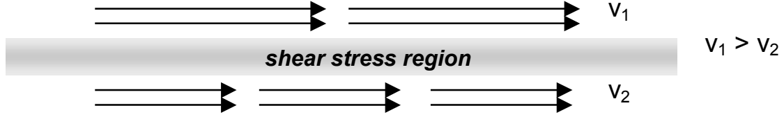
Figure 2-6. Viscous losses in a fluid. A shear stress and losses can be originated by differences of the particle velocities at neighboring regions in the fluid.
