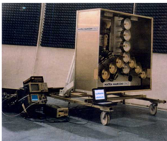
Figure 1.1. The MIRAS demonstrator, operated by the European Space Agency in order to demonstrate the potential for a future space borne L-band radiometer.
