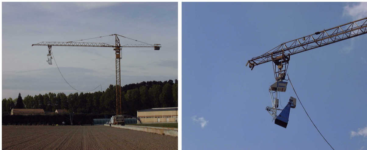
Figure 5.2. The radiometer installation at Institut National de la Recherche Agronomique, Avignon, France. The EMIRAD L-band radiometer is mounted on the crane, 20 m above the cornfield. Incidence angles vary from 0 to 60^\circ , and azimuth angles from -90^\circ to 90^\circ .
