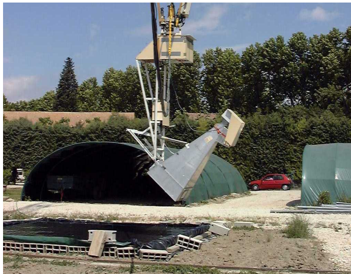
Figure 5.6. The 6 m by 6 m calibration pool used for evaluation of the long term radiometer stability during the 2001 Avignon experiment.
