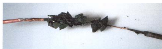
Figure 2 Copper wire after one week in a concentrated THF solution of 1 . Notice how thin the copper wire is in the middle compared to the ends, and how the crystals of the cis -[di( N,N -diethyl(2-phenyldiazanyl)thioformamide-κS,κN 2 )]copper ( 5 ) are growing on the wire.
