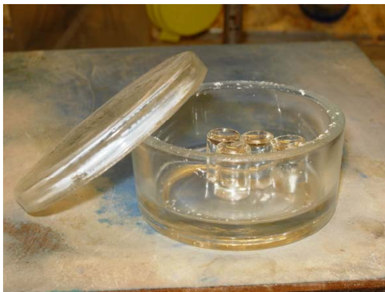
Figure 31. The equipment for the sitting-drop vapor diffusion technique.
