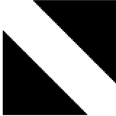
Figure 8.2: Prior field to illustrate the problems associated with the use of gradients in structural modeling. Compared to the field shown in Figure 8.1 the connectivity to the well in the lower left corner is not present.
