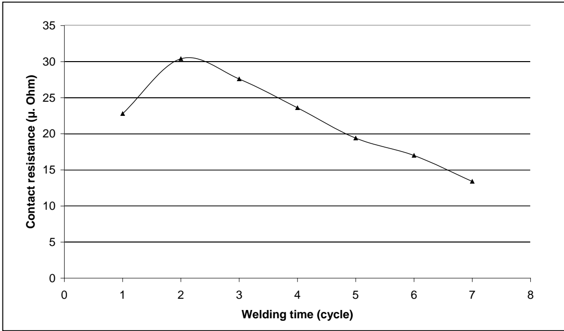
Fig. 8.5 — Faying surface contact resistance of mild steel
