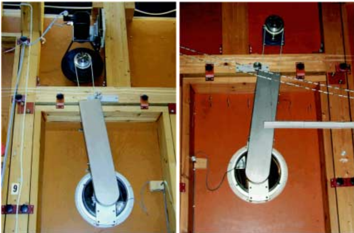
Figure A.4: One servo, shown in the upper part of the left figure, drives the 1DOF movement mechanisms on both sides using a shaft on top of the wind tunnel. This ensures that the phase-difference between the motion on the two sides of the tunnel is kept very low.
