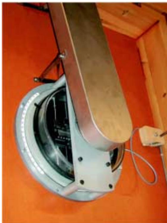
Figure A.7: A plexiglass cover encloses the movement mechanism to prevent air from leaking into the tunnel during operation of the wind tunnel. Outside tunnel view.
