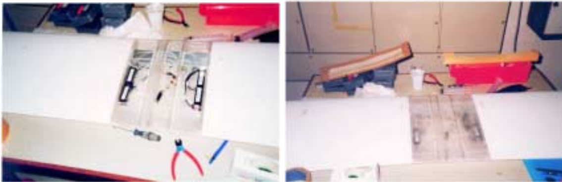
Figure A.1: The pressure transducers were located inside the airfoil test section to minimize the length of the tubes connecting the pressure taps to the transducers. The orientation of the transducers were such that the fictitious forces from the motion of the airfoil had identical effect on all transducers, thus cancelling out in the computation of lift, drag and moment. Note the hollow rectangular aluminum beam at the quarter-chord, which provides the stiffness to the model .
