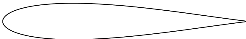
Figure C.1: 15 % thick Van de Vooren airfoil with a trailing angle \tau = 12.5^\circ .
