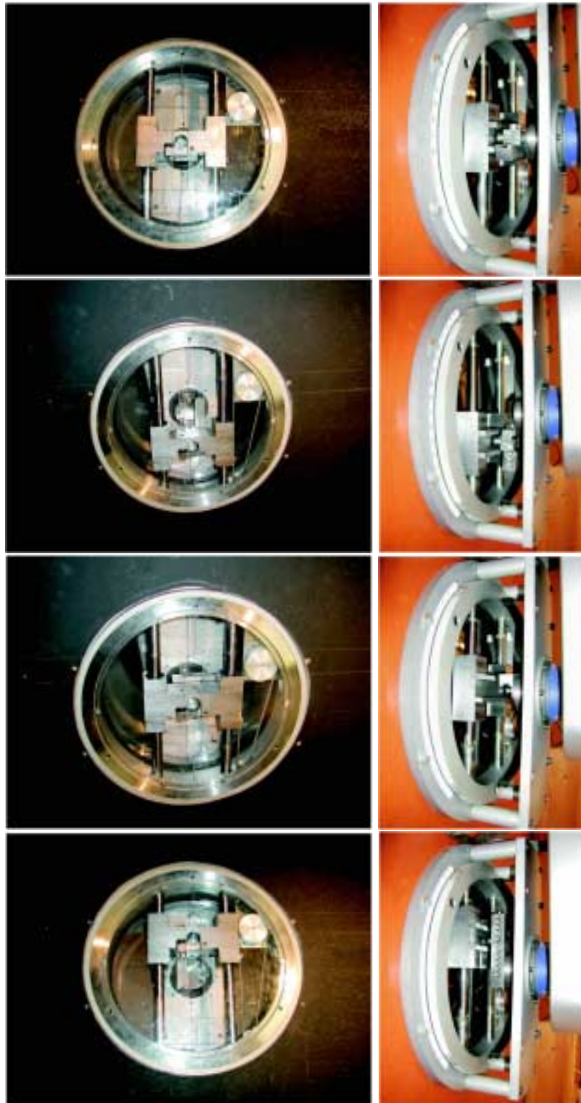
Figure A.5: Movement mechanism for the 1DOF translatory motion shown at four different stages of the rotational cycle. Left figures: View from inside of the wind tunnel. Right figures: View from the outside of the tunnel.
