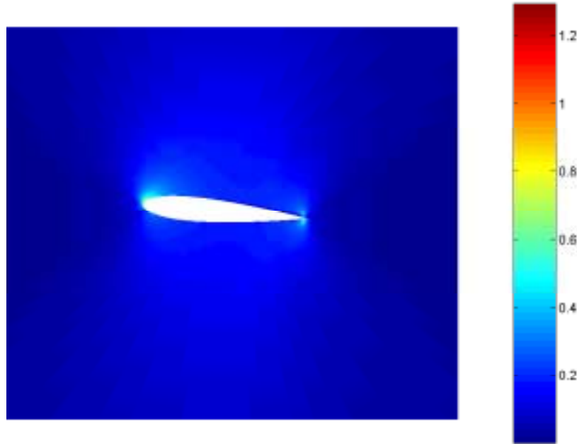
Figure 4.28: CFL-number for the solution of the flow around the NACA 0015 airfoil at Reynolds number Re = 555000 . The incidence is \alpha = 5^\circ .
