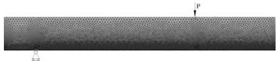
Figure 8. FE-mesh for the fully symmetric domain. The left half of the beam is modeled.
