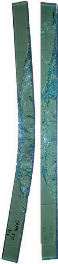
Figure 6. Beams after test. left: 3 mm steel reinforcement, the crack patterns are similar to what is seen in concrete. right: 6 mm steel reinforcement, failure when delaminating in the adhesive layer.
