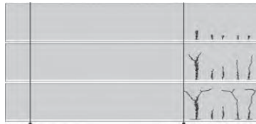
Fig. 14: Plot of cracked elements for three different relative midpoint deflections. Top: Circle 1; middle: Circle 2; bottom: Circle 3. The vertical line to the left represents the support and the vertical line to the right represents the position of load application
