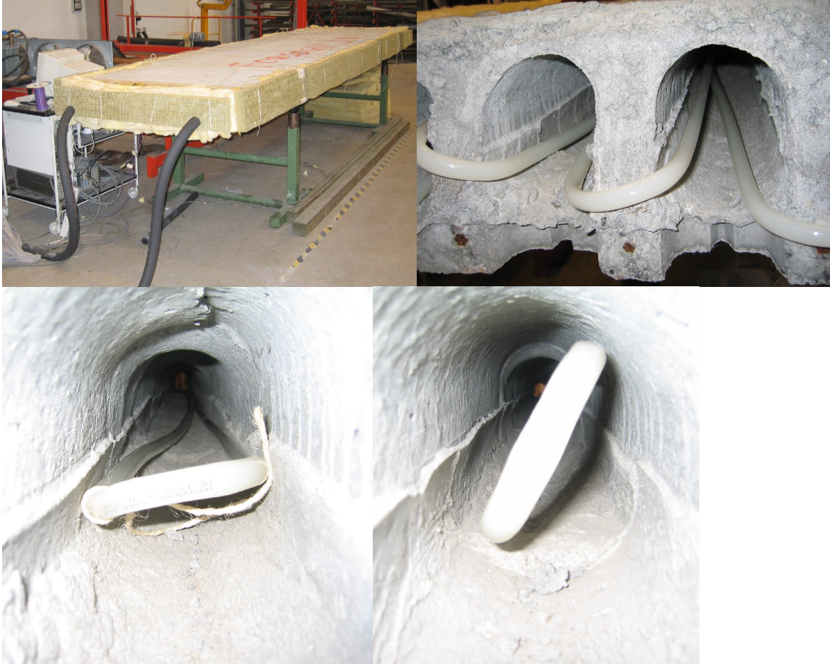
Figure 6.7 Pictures of setup. The upper left picture shows the deck during testing. The deck is insulated to the sides and ends. The upper right picture shows the bend of the pipe in the end where it leaves one cavity to enter the next. The lower pictures show two examples of the pipe position at the far end of the deck. The bends are approximately 10 cm from the end of the deck.
