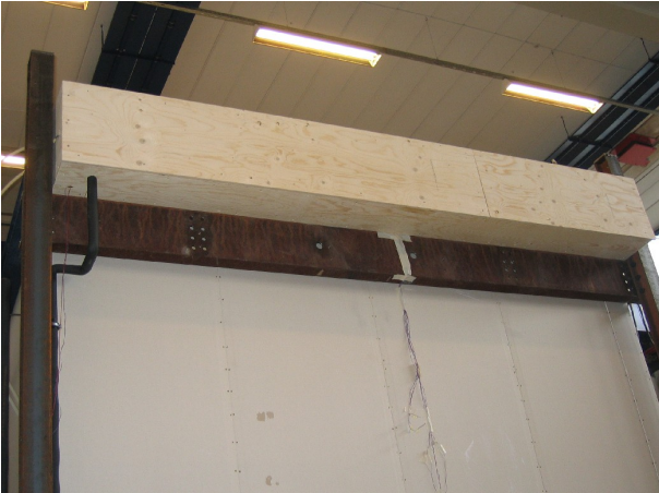
Figure 6.19 End of upper deck after being finished. The wooden box is filled with insulation thereby minimizing the unwanted heat loss from end of deck and manifold. All four deck ends (upper and lower) have the same insulation box.
