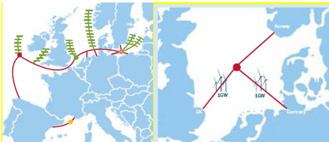
Figure 4: The SuperNode configuration could be a first step for the development of the European Supergrid. It would allow the three-way trading of power between the UK, Norway and Germany, and include two 1 GW offshore wind farms, one in the UK and one in Germany. Depending on the wind farm output at any given time, the capacity for trade would go up to 1 GW between each pair of countries in the combination 13 .
