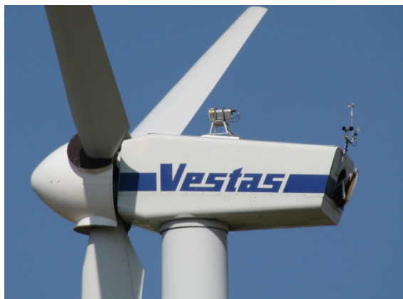
Figure 1 ZephIR lidar's optical head mounted on the V27 wind turbine's nacelle.
