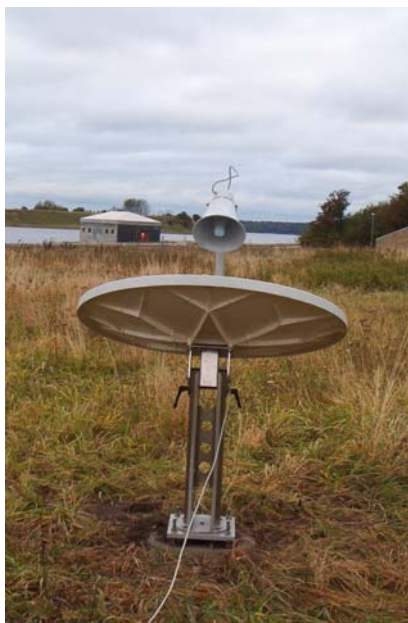
Figure 1. The Heimdall sodar transmitter at Risø. The speaker is located in the focus of the antenna disk.
