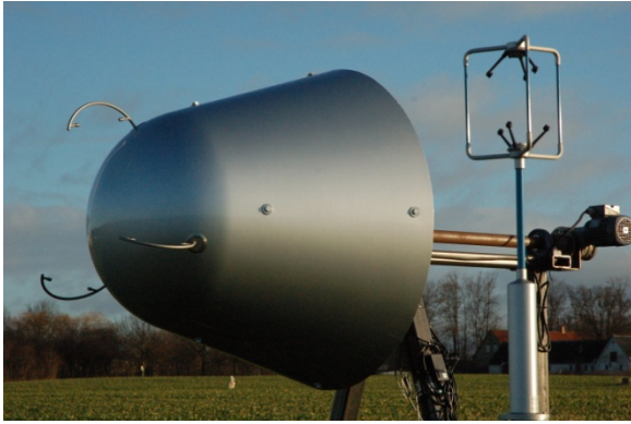
Figure 6 Arrangement of the S300 spinner anemometer with "new" sensors in comparison with the sonic anemometer at Risø test site
