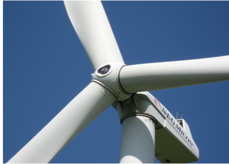
Figure 1 Photograph of the NM 80 wind turbine. Here it is visible the optical head of the QinetiQ's (Natural Power) ZephIR lidar in the tip of the wind turbine spinner (left). In addition it can be seen the interior of the spinner were the lidar was mounted (right).
