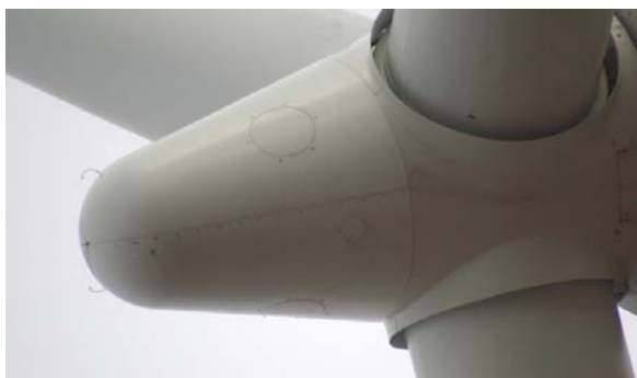
Figure 10 The three 1D sonic wind sensors mounted on the 3,6MW wind turbine spinner at Risø DTU Høvsøre test site.
