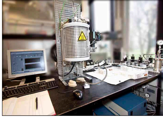
Fig. A.6: Setup for testing the catalytic SCR activity at various temperatures. \text{NH}_3 - \text{NO}_x -analyzer located below table along with gas diluting unit
