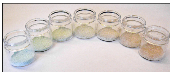
Fig. A.2: Fe-Cu mixed oxide catalysts supported on 3.4SZ_NP. From left to right decreasing copper oxide loading, increasing iron oxide loading
