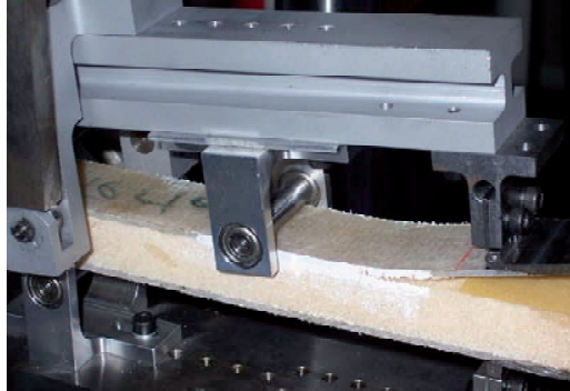
Fig. 4. Observed crack propagation path in a MMB specimen during testing, with crack growth in the core.
