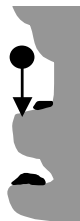
Figure 3.11: The dominating force on large particles is gravity; the downward force causes settling of particles. At vertical rough surfaces particles will settle at projections.
