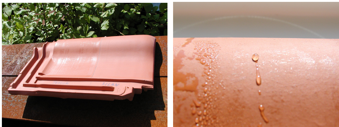
Figure 6.2: Left: an ordinary tile treated with "Teflon" (left) and silan (right). "Teflon" gave the tile a glossy look. Right: Water at "Teflon" formed an almost perfect spherical droplet.
