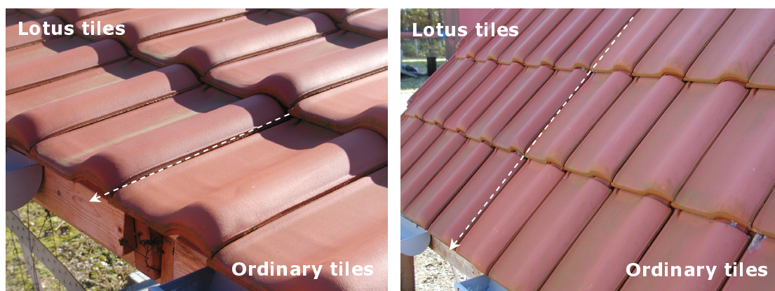
Figure 5.3: Soiling of north faced surfaces after 28 month. To the left in each picture are tiles with Lotus Effect, to the right ordinary tiles (separated through a dashed line). In the picture of low sloped roof (left-hand picture) the soiling forms a distinct stripe, while the overall impression is, that tiles with Lotus Effect soil, but at a somewhat slower rate than ordinary tiles.
