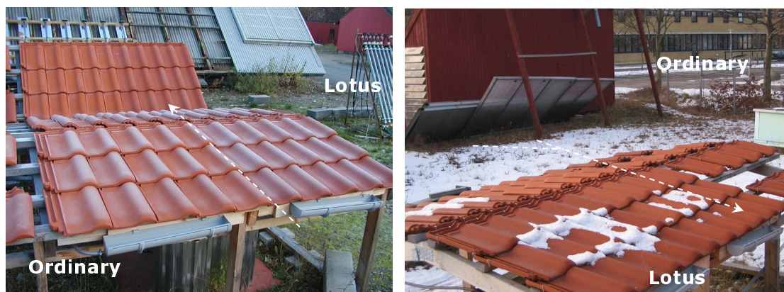
Figure 5.27: Difference in thermal behaviour of tiles with and without Lotus Effect. Left: rimy tiles, the tiles with Lotus Effect (right side) were whiter than the ordinary tiles. Right: melting snow, the snow melts off faster from ordinary tiles (right side).
