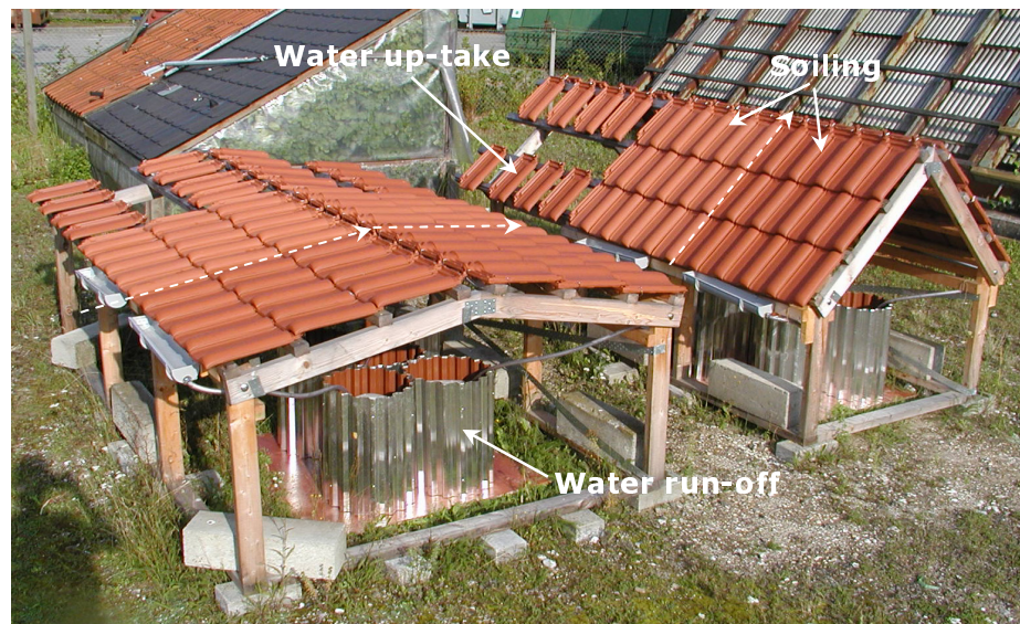
Figure 5.7 The set-up used for soiling and wetting tests. For the soiling and water run-off tests three rows with 5 tiles with and 5 tiles without Lotus Effect were placed in different slopes ( 12^\circ and 45^\circ ) and two orientations (north and south). Gutters were placed under the central tiles in each set-up, and the water was collected in plastic containers, here hidden by metallic sunscreens. Tiles for weighing were placed at the same frames and can be seen in the back as two rows of 4 individually tiles.
