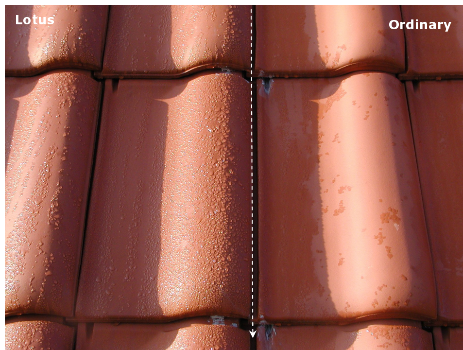
Figure 5.23: Dew at tiles. Left: Dew forms droplets at tiles with Lotus Effect. Right: Dew is only visible as a film on ordinary tiles or has already dried up.
